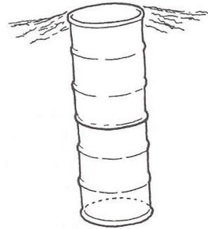
The small volume and the high cost of the drums make this method fairly expensive. If the sides of the drums are not provided with sufficient perforations, absorption of liquids can be a problem. Another problem is that the sheet metal will eventually corrode and collapse if the drums are too old.
